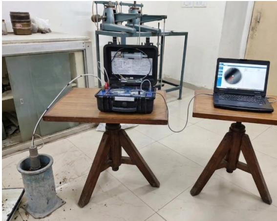
Fig-2: Lab Flat Dilatometer Test Setup
