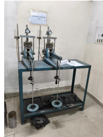
Fig-3: Oedometer Consolidation Test Setup
