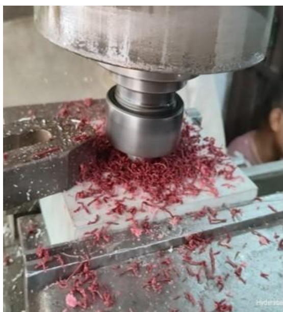
Fig.3. FSE process setup on milling machine
