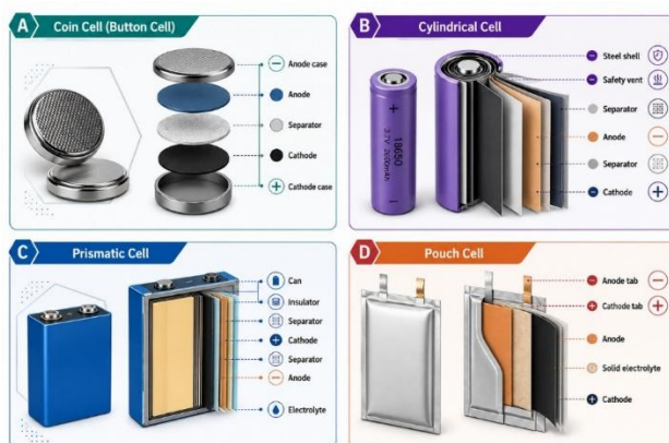
Figure 5: The AI picture of common configurations of rechargeable batteries: (A) coin, (B) cylindrical, (C) prismatic, and (D) pouch
