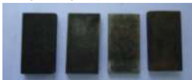
Fig. 3.1 Specimen for abrasive wear rate analysis and hardness testing
