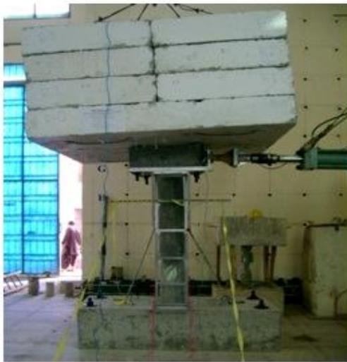
Fig. 1. Scaled RC bridge columns
