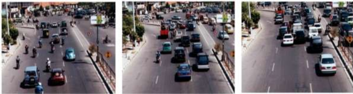
Fig 1. The queue is built up during red signal in mixed traffic conditions
