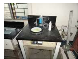
Fig: 3.4 – Fine polisher equipped with a rotating wheel covered with polishing cloth
