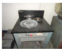
Fig: 3.3 – Coarse polisher equipped with a rotating wheel with fine emery paper
