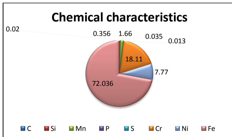
Fig 4. Chemical characteristics of work piece SS 202
