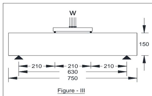
Figure-III Details of test beam
