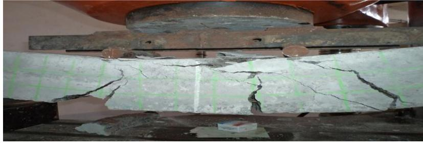
Figure-IV Failure of DSSR Beam-1
