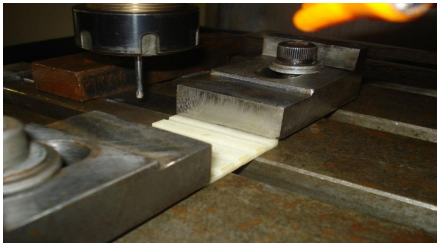
Figure 3. Fixation of GFRP composite plate by using clamps in the machining centre
