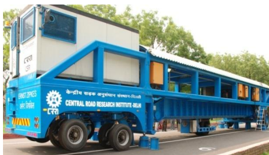
Fig 2: HVS(APTF) Operating at CSIR-CRRI
