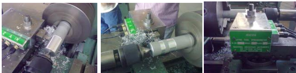
Fig 4: Turning process, testing under way and Lathe Tool Dynamometer
