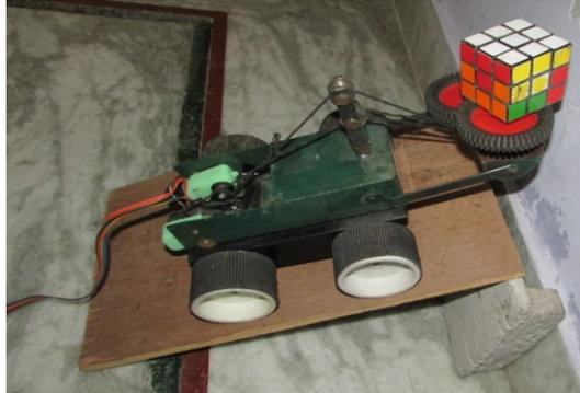
Observation shows that by making it differential drive we can reduce its turning radius as compared to conventional steering mechanism and this helps in better controlling and operating the backhoe loader. Hence ergonomics study confirms that by adopting this type of mechanism in a backhoe loader, we can significantly reduce the chances of an accident while the operator is performing an operation.
