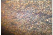
Image 3b.Micro structure of LM25 with 10% Al<sub>2</sub>O<sub>3</sub> and 3% Flyash
