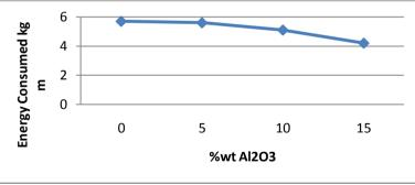
Fig:3.4.1 Impact load absorption(In kg m) with % wt Al2O3
