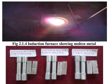
Fig 2.1.5 Tensile and impact test specimen with varying composition of Al<sub>2</sub>O<sub>3</sub>
