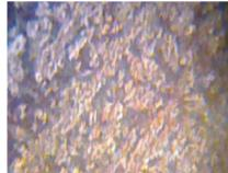
Image 3a.Micro structure of LM25 with 5% Al2O3 and 3% Flyash
