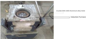
Fig.2.1.1 Induction furnace with Crucible containing LM25
