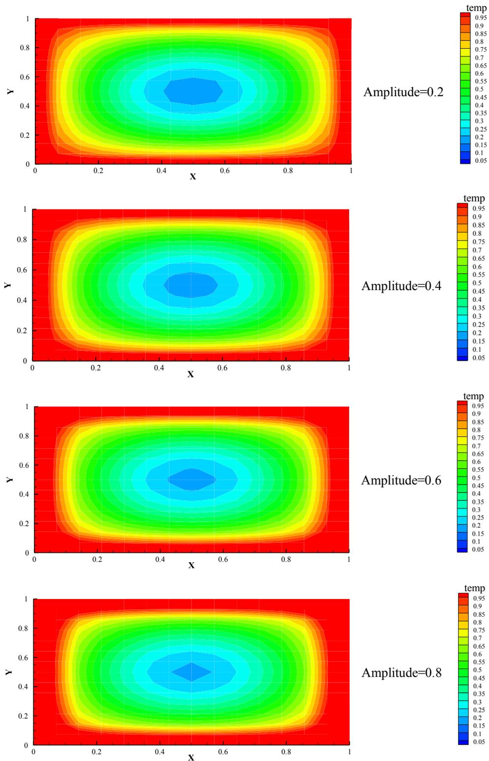
**fig. (8): three dimensional transient temperature distribution of different amplitude at section ( $z=0.35$ ) for  $Ra=200$ , period=0.01,  $t=0.024$**
