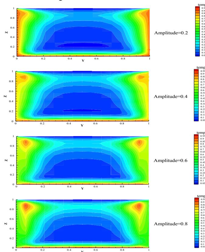
**fig. (3): three dimensional transient temperature distribution of different amplitude at section ( $x=0.214$ ) for  $Ra=200$ , period=0.01,  $t=0.006$**
