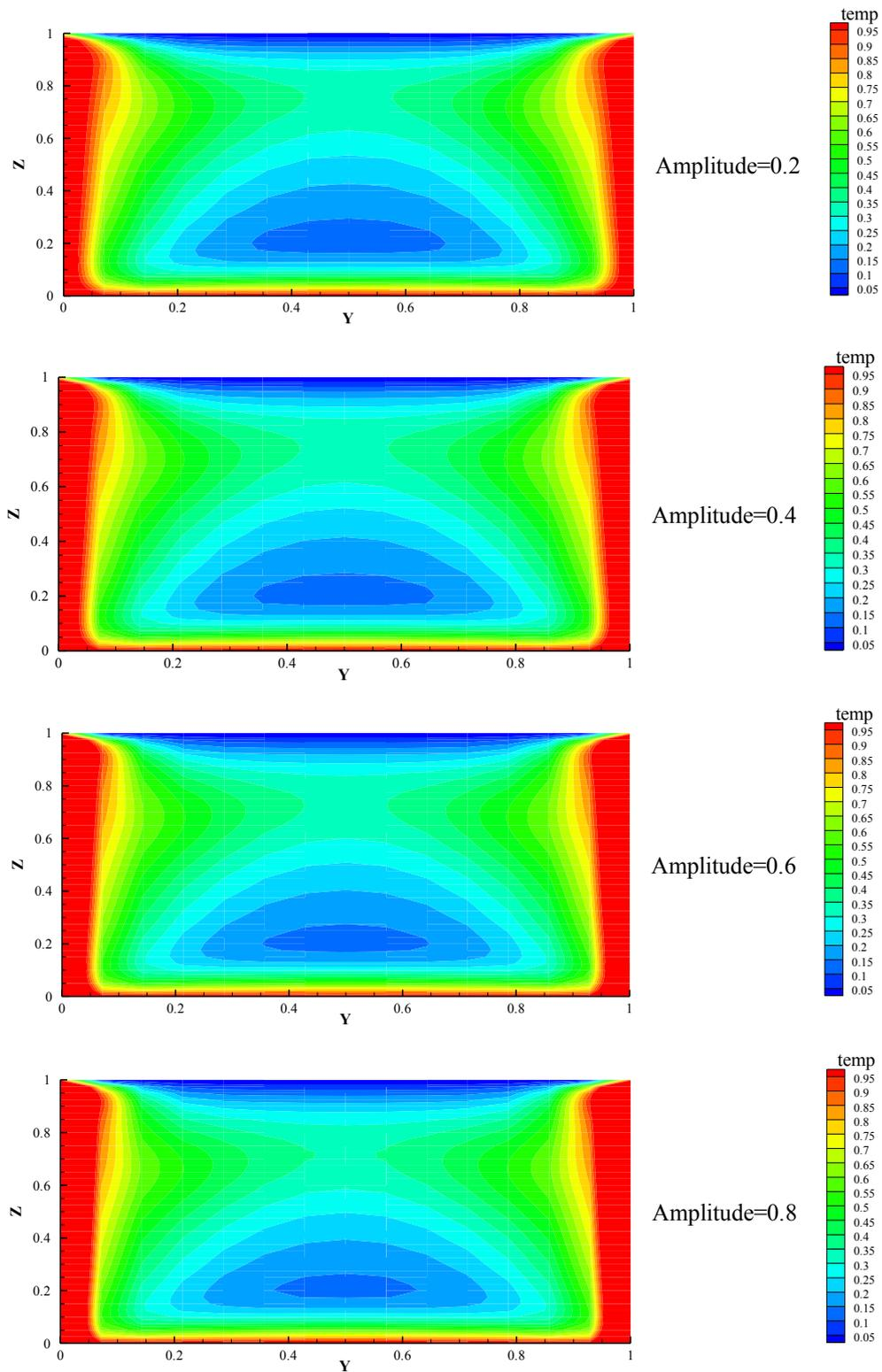
**fig. (5): three dimensional transient temperature distribution of different amplitude at section ( $x=0.214$ ) for  $Ra=200$ ,  $period=0.01$ ,  $t=0.012$**
