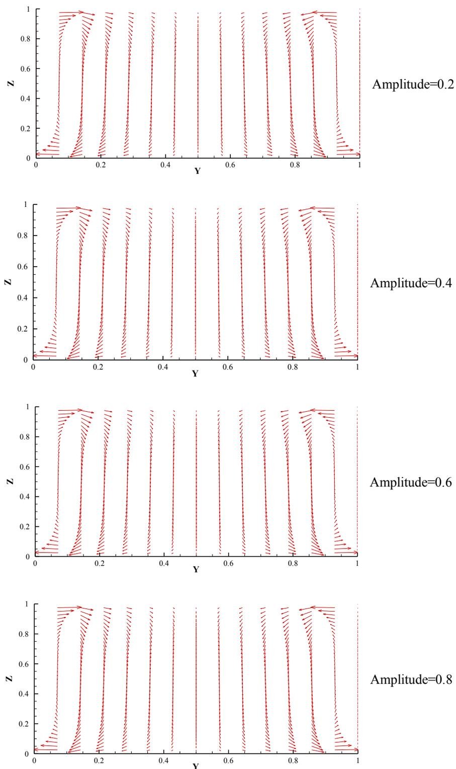
**fig. (9): velocity distribution of different amplitude at section ( $x=0.214$ ) for  $Ra=200$ , period=0.01,  $t=0.006$**
