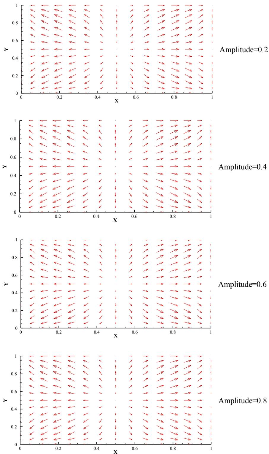
**fig. (12): velocity distribution of different amplitude at section ( $z=0.35$ ) for  $Ra=200$ , period=0.01,  $t=0.024$**
