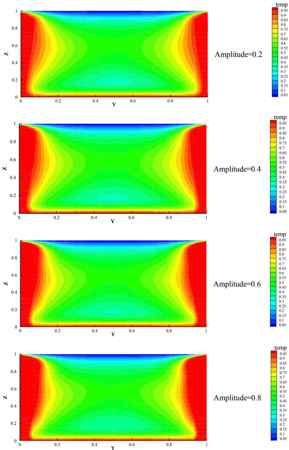
**fig. (7): three dimensional transient temperature distribution of different amplitude at section ( $x=0.214$ ) for  $Ra=200$ ,  $period=0.01$ ,  $t=0.024$**
