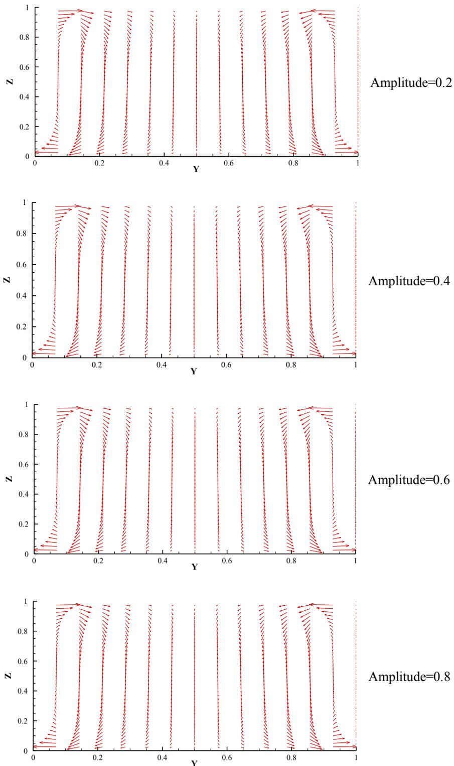
**fig. (11): velocity distribution of different amplitude at section ( $x=0.214$ ) for  $Ra=200$ , period=0.01,  $t=0.024$**
