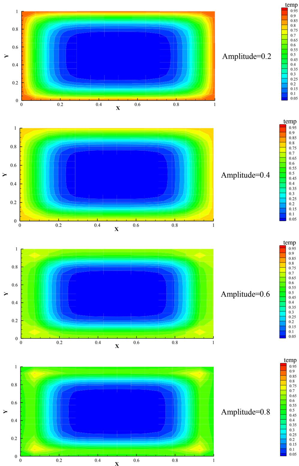
**fig. (4): three dimensional transient temperature distribution of different amplitude at section ( $z=0.35$ ) for  $Ra=200$ , period=0.01,  $t=0.006$**
