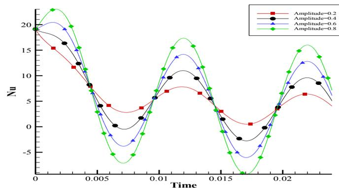
fig.(13): variation of Nusselt number with time at the vertical wall for various values of amplitude
