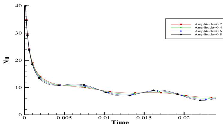
fig.(14): variation of Nusselt number with time at the bottom wall for various values of amplitude
