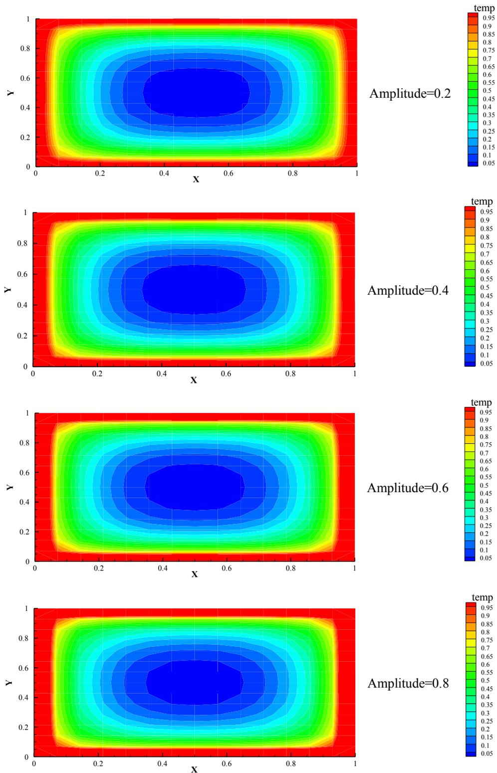
**fig. (6): three dimensional transient temperature distribution of different amplitude at section ( $z=0.35$ ) for  $Ra=200$ , period=0.01,  $t=0.012$**
