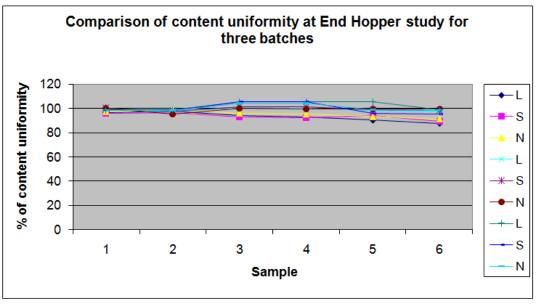
Trend chart for content uniformity at end Hopper study for three batches
