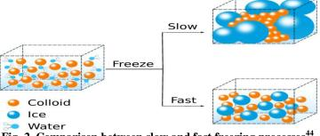
Fig. 2. Comparison between slow and fast freezing processes<sup>44</sup>
