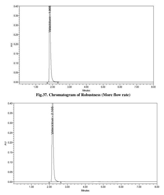
Fig.38.Chromatogram of Robustness (Less Flow rate)
