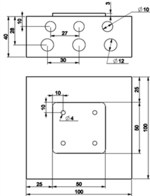
Figure 1. Dimensions of the mold plate
