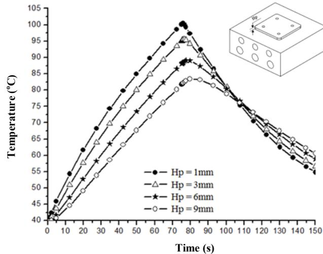
**Figure 8.** Simulation result of mold temperature history for different product heights.
