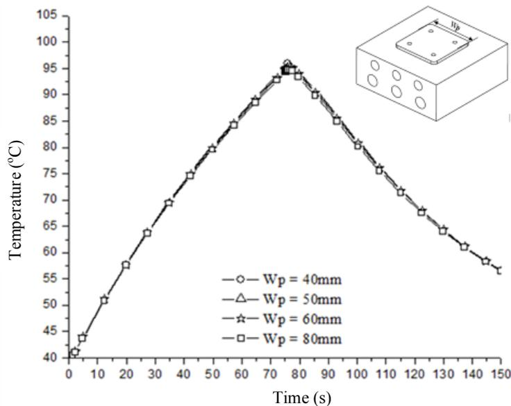
Figure 5. History of mold temperatures with different product widths.
