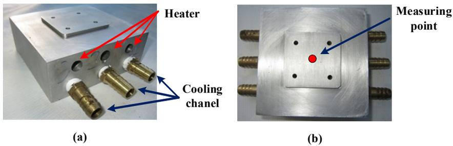
Figure 4. Experiment model with the side view (a) and top view (b)
