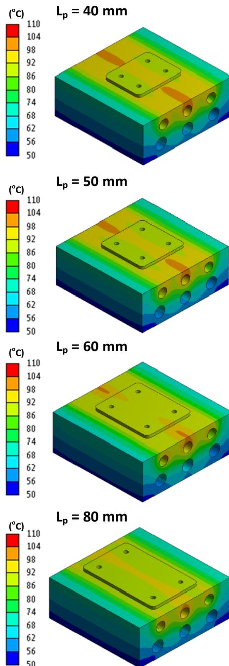
**Figure 6.** Mold temperature distribution with different product lengths.
