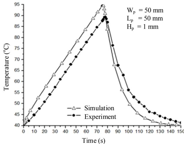
**Figure 9.** Mold temperature comparison between simulation and experiment results
