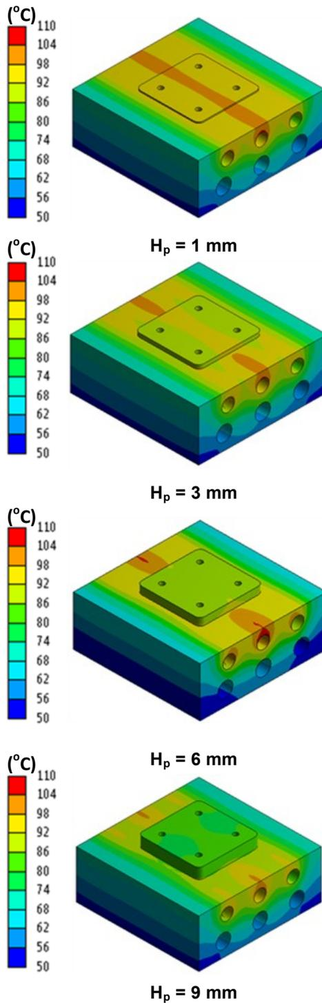
Figure 7. Mold temperature distribution with different product heights.
