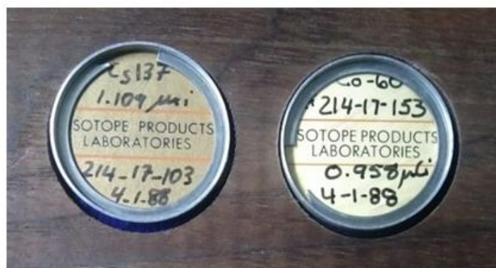
Figure no 1: Gamma radioactive point sources ^{137}\text{Cs} & ^{60}\text{Co}
