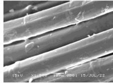
Picture no11: Results of SEM Analysis on Ramie Fabric After Modification (a)Inside the surface of ramie fiber (b)On the surface of ramie fiber
