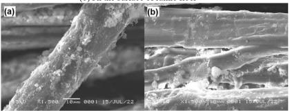
Picture no12: Results of SEM Analysis on Ramie Fabric After Washed (a)Inside the surface of ramie fiber (b)On the surface of ramie fiber
