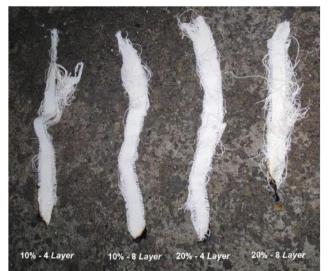
Picture no7: Results of Washing Evaluation on Ramie Fabric After Modification
