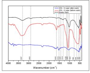
Picture no9: Results of FTIR Characterization on Ramie Fabric Before and After Washed
