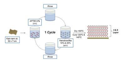
Picture no1: Illustration of Layer by Layer Methods on Ramie Fabric-APTES-Nanobiosilica
