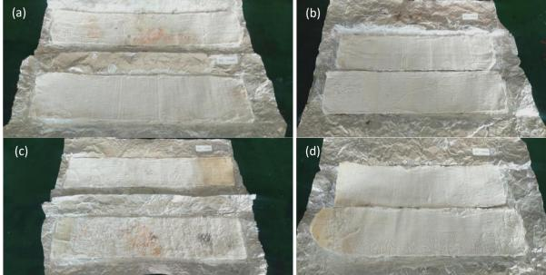
Picture no3 shows the results of weighing ramie fabric before and after modification using NBS using the Layer by Layer method. Here, it can be seen that the post-modified fabric does not always show an increase in fabric weight even though the number of layers applied is increased. This can happen because when ramie fabric is rinsed after being soaked in the NBS solution, some of the NBS that has previously adhered to the fabric is released.
