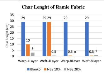
Picture no5: Char Length Graphs of Ramie Fabric Before and After Modification
