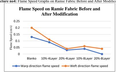
Picture no4: Flame Speed Graphs on Ramie Fabric Before and After Modification
