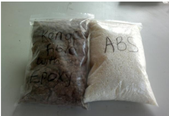
Figure1a: The epoxy treated kenaf fibre and ABS thermoplastic.
