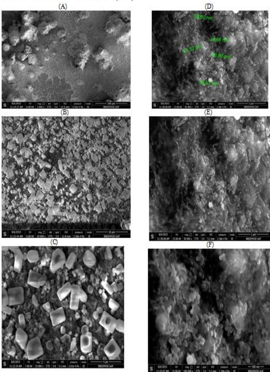
Figure 3. Scanning Electron Micrograph of Chitosan-alginate-hydroxy apatite Nanocomposites (A-F).
