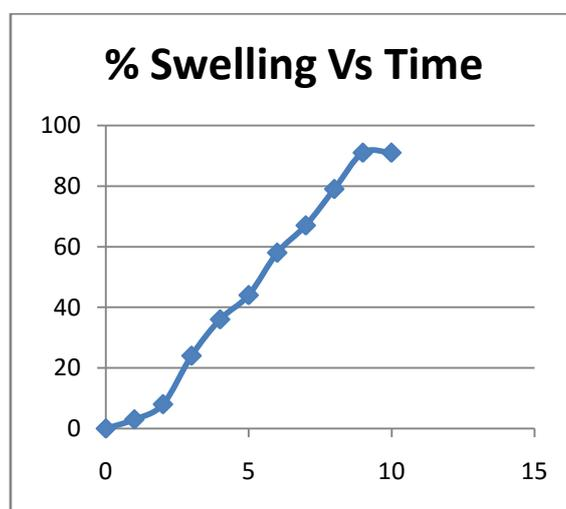
Figure 7. Water Absorption of the chitosan-sodium alginate nanocomposites
