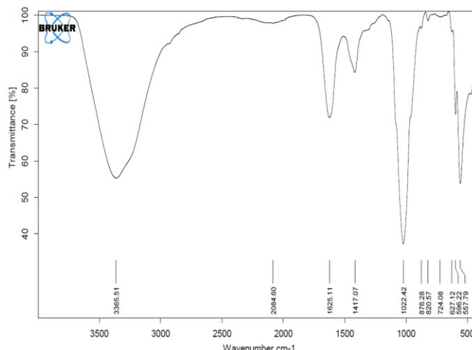
**Figure 1.** FTIR-Spectra of chitosan Alginate hydroxyl apatite nanocomposite.
