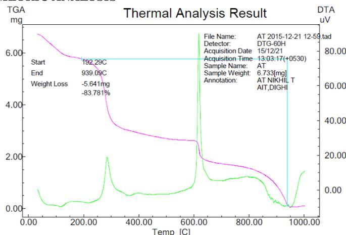
Fig. 6: Thermogravimetric analysis of nanocomposite.
