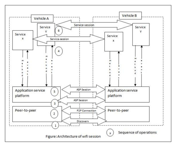
In the figure the real time scenario is explained. At first whenever two vehicles will be in close range, there will peer-to-peer discovery. Then P2P connection will be established. ASP session would be created which will be responsible to provide session for microcontroller which will measure the distance of two nearby vehicles.
