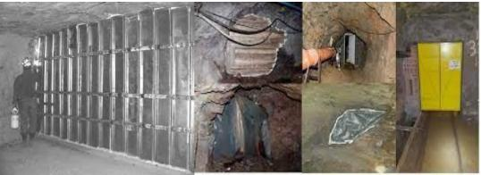
Figure 9: Mine Ventilation Stopping (Source: cdc.gov and researchgate.net)
