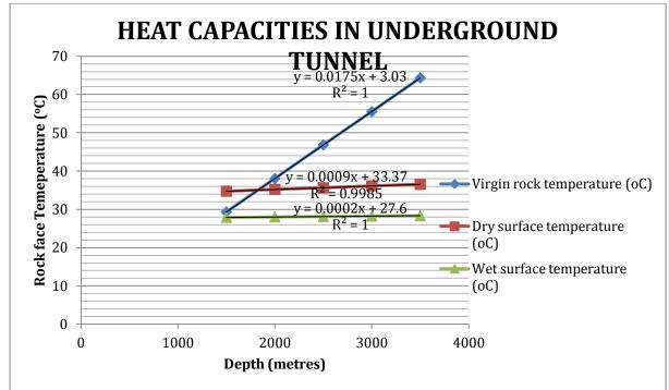
Figure 3: Heat Capacities in Underground Tunnel
