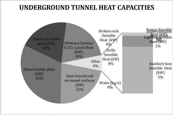
Figure 4: Underground Tunnel Heat Capacities
