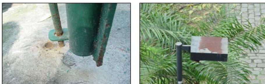
Figures 15, 16 – Atmospheric corrosion of rod and box of carbon steel.
