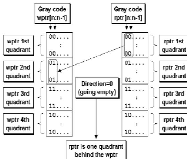
Figure 3.FIFO is going empty because the rptr trails the wptr by one quadrant
