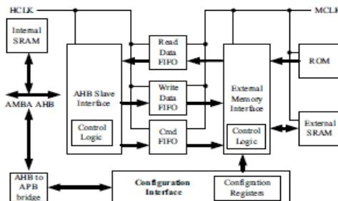
Figure 10.Architecture of AHB-MC
