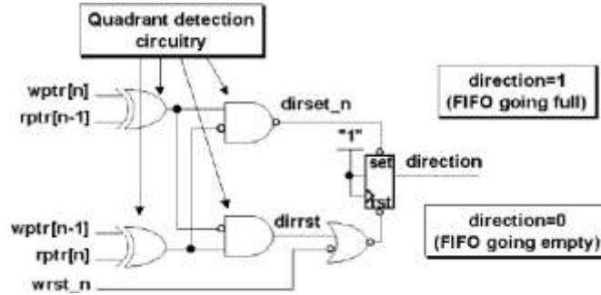
Figure 4.FIFO direction quadrant detection circuitry
