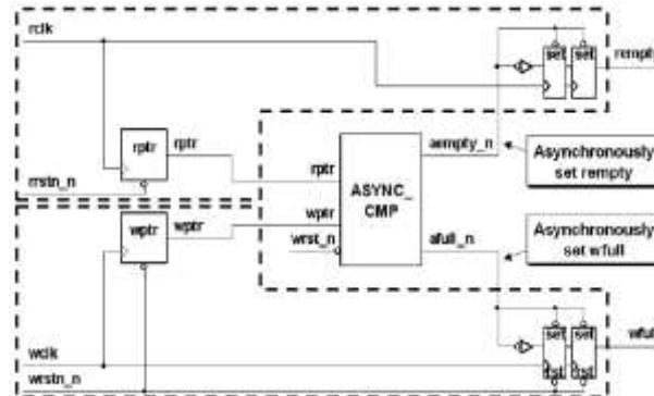
Figure 7.async\_cmp module connection to rptr\_empty and wptr\_full modules.
