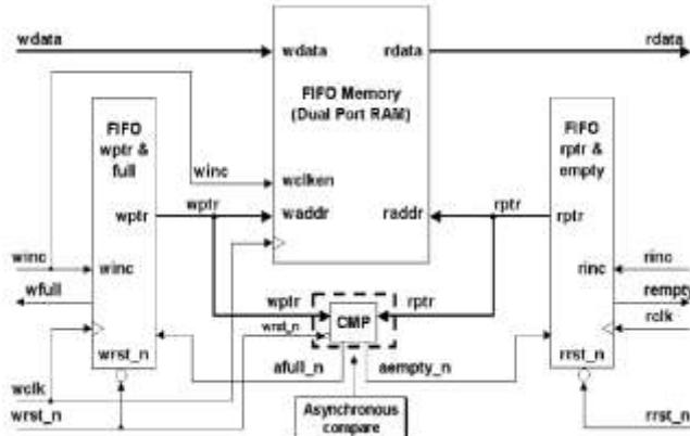
Figure 5. FIFO2 partitioning with asynchronous pointer comparison logic
