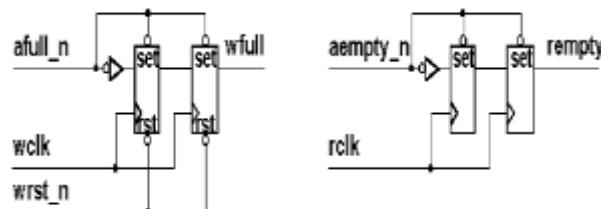
Figure 8 .Asynchronous empty and full generation
