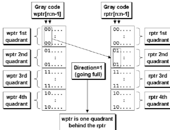
Figure.2: FIFO is going full because the wptr trails the rptr by one quadrant If the write pointer is one quadrant behind the read pointer, this indicates a "possibly going full" situation as shown in Fig: 2. When this condition occurs, the direction latch of Figure 4 is set.
