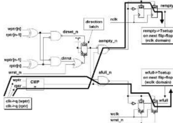
Figure 9 .Critical timing paths for asserting rempty and wfull.
