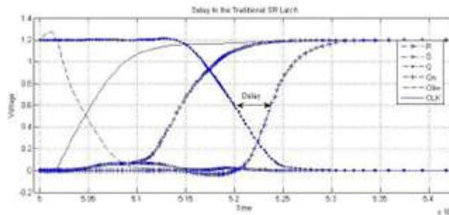
Fig.3: Delay between Q and /Q of SR Latch
