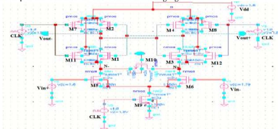
Fig.1: Conventional Sense Amplifier Based Comparator
