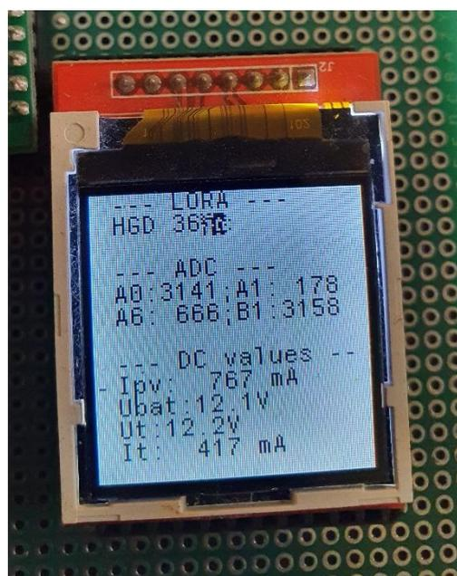
Figure3. Screen shows the operation variables of the system (I<sub>pv</sub>: current from solar panel, U<sub>bat</sub>: voltage of battery, U<sub>t</sub>: load voltage, I<sub>t</sub>: load current)
