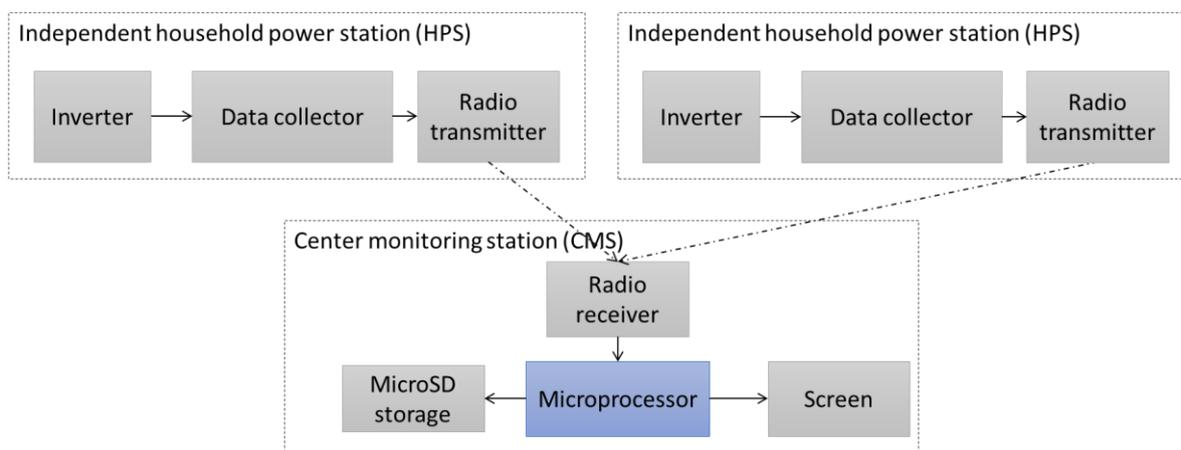
**Figure1.** System diagram
