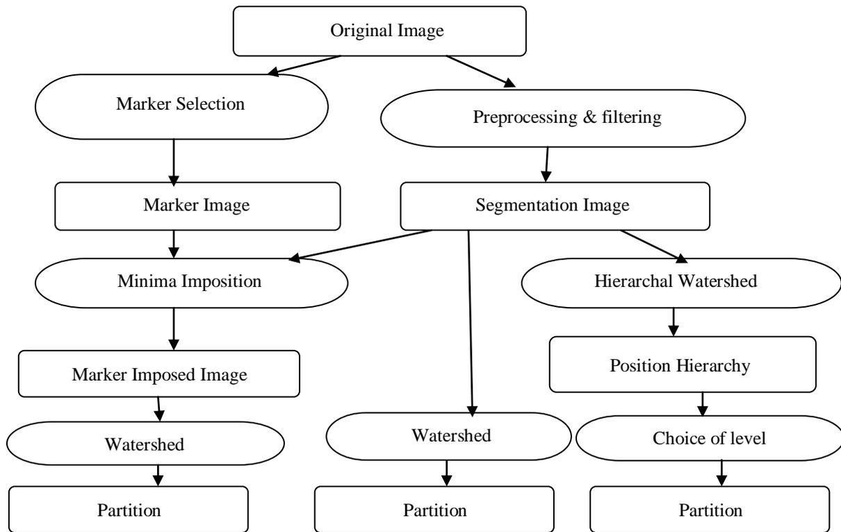
Fig 1. Three approaches in watershed segmentation
