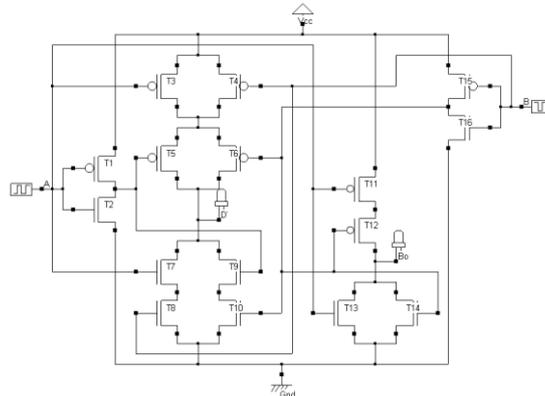
Figure 3 – Transistor level Half-Subtractor Circuit
