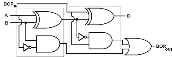
Figure 1 – Logic Symbol of Full-Subtractor
