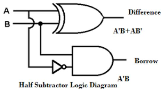
Figure 2 – Logic Symbol of Half-Subtractor
