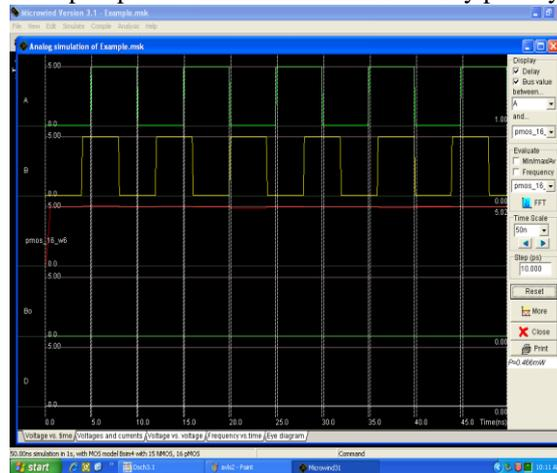
Figure 8 – Waveform of conventional Half-Subtractor
