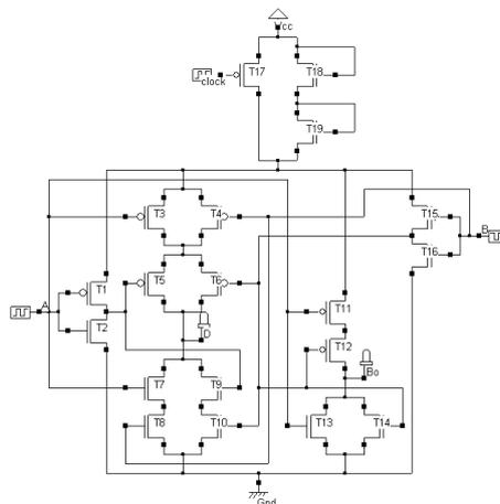
Figure 6 – Half Subtractor using AVLS Technique
