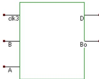
Figure 5 – Logic Symbol of the Half-Subtractor using AVLG Technique
