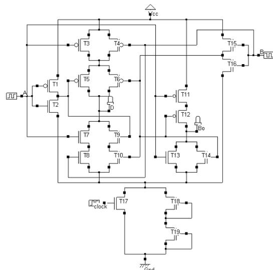
Figure 4 – Half-Subtractor using AVLG Technique
