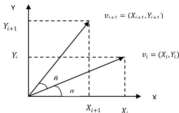
Fig (1) A 2D vector rotation using CORDIC
