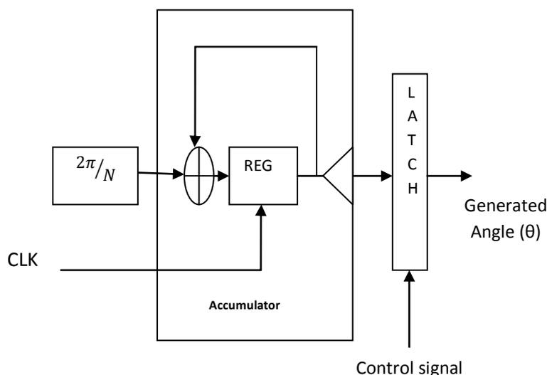
Fig 3  $\theta$ - generator of the proposed system.
