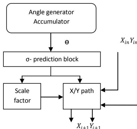
Fig 2 Block schematic of the proposed system
