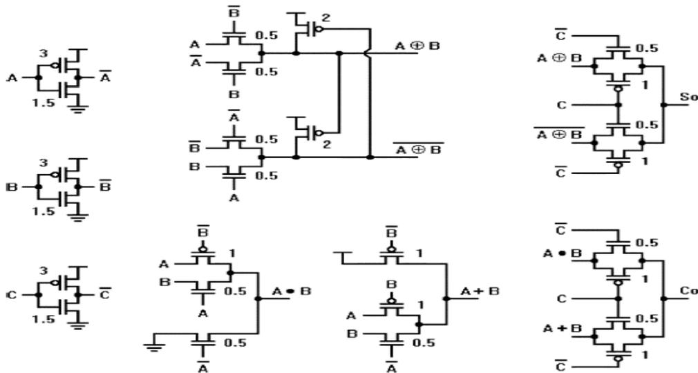
Figure 3: Full-Adder designed with the Existing logic Structure and a SR-CPL Logic Style.
