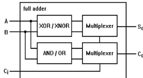
Figure 1: Alternative logic scheme for designing full-adder cells.
