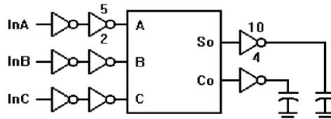
**Figure 7: Test bed used for simulating the full-adders under comparison**
