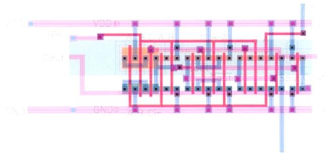
Figure 8 Layout of ripple carry adder
