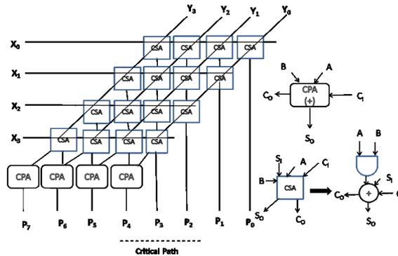
Fig 5.6 Architecture of 4 bit multiplier
