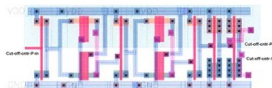
*Figure 12 Layout of the control signal Shifter for remaining clusters.*
