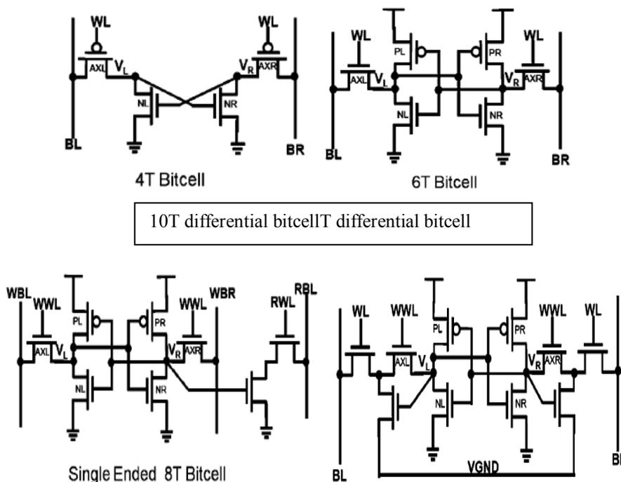
**Fig.1 different bitcell configurations**
