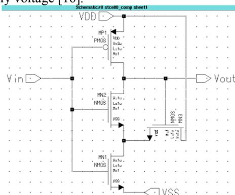
**Fig2. Basic Schmitt trigger bitcell**
