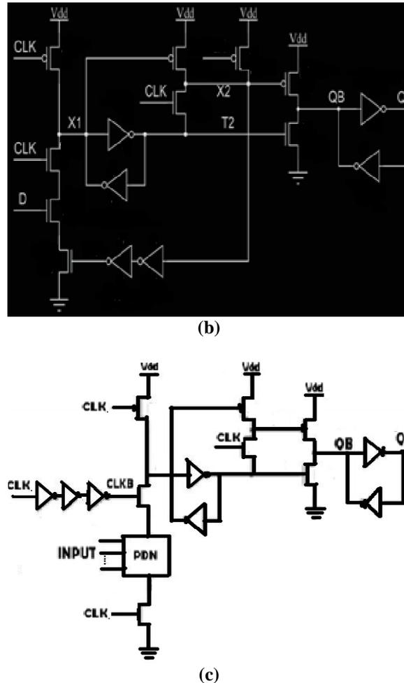
Fig. 1 Schematic view of Flip-flop topologies analyzed (a) XCFF (b) DDFD (c) DDFD-ELM
