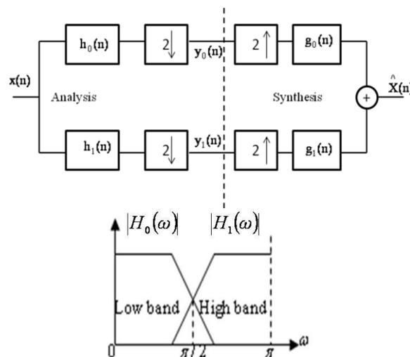
Fig 3. Two-band filter bank for one-dimension subband coding and decoding.
