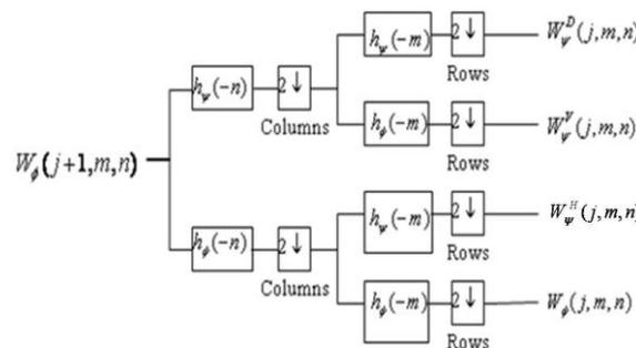
Fig 5. The two-dimensional FWT – the analysis filter bank
