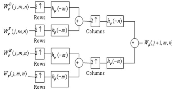
Fig 7. The two-dimensional DWT – The synthesis filter bank
