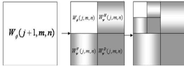
Fig 6. Two-Scale of Two –Dimensional Decomposition
