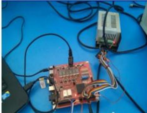
Figure 7: Hardware implementation on FPGA
