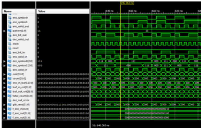
Fig. 11: Simulation wave forms for decoding of Convolutional codes.
