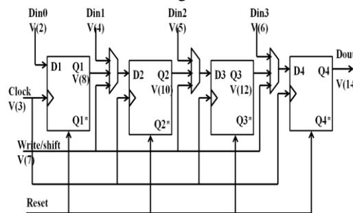
Fig 9. Parallel-in and Serial-out shift register.
