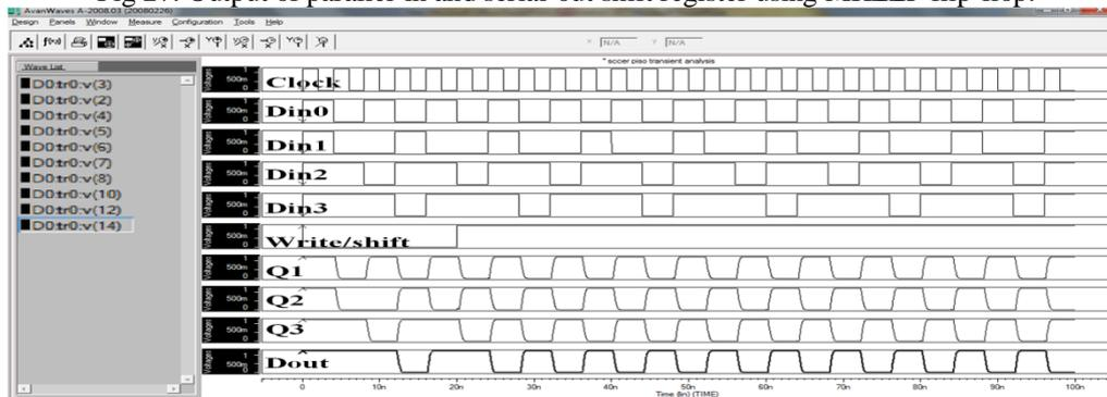
Fig 28. Output of parallel-in and serial-out shift register using SCCER flip-flop.
