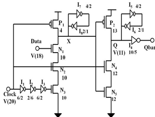
Fig. 2. Circuit Diagram of IP-DCO Flip-Flop.
