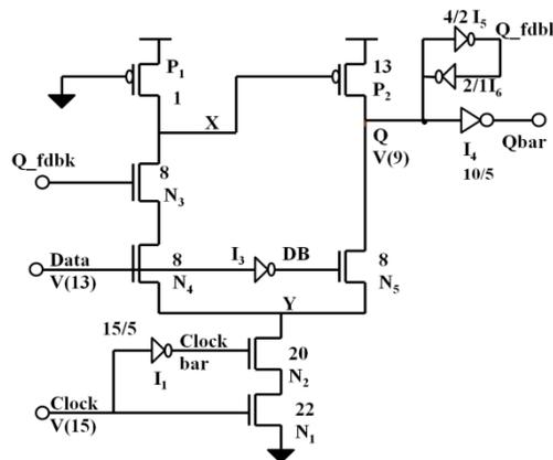
Fig. 4 Circuit Diagram of SCCER Flip-flop.
