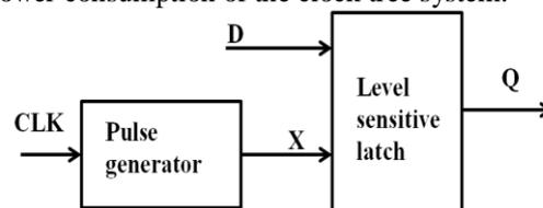
Fig 1. Block diagram of a pulse triggered Flip-flop
