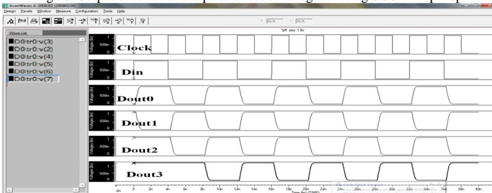
Fig 21. Output of serial-in and parallel-out shift register using proposed flip-flop.
