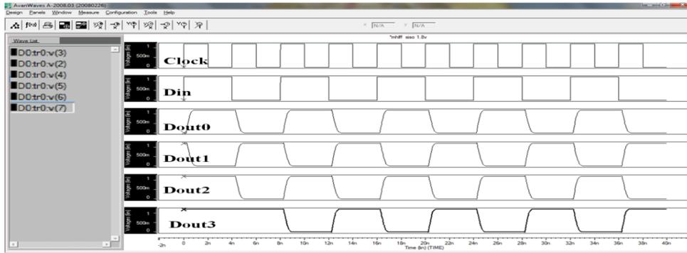
Fig 19. Output of serial-in and parallel-out shift register using MHLFF flip-flop.
