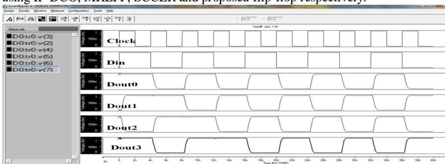
Fig 18. Output of serial-in and parallel-out shift register using IP-DCO flip-flop.
