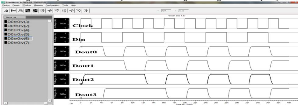
Fig 20. Output of serial-in and parallel-out shift register using SCCER flip-flop.
