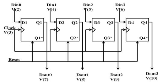
Fig. 8 Parallel-in and Parallel-out Shift Register.
