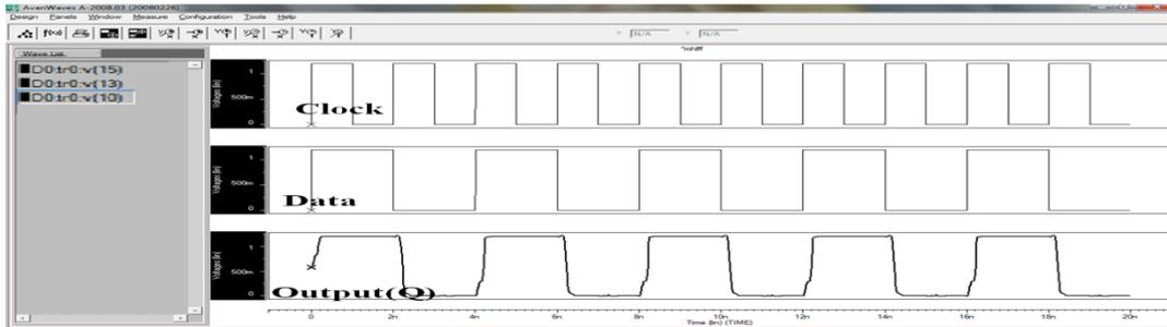
Fig 11. Output of Modified Hybrid Latch Flip-flop.
