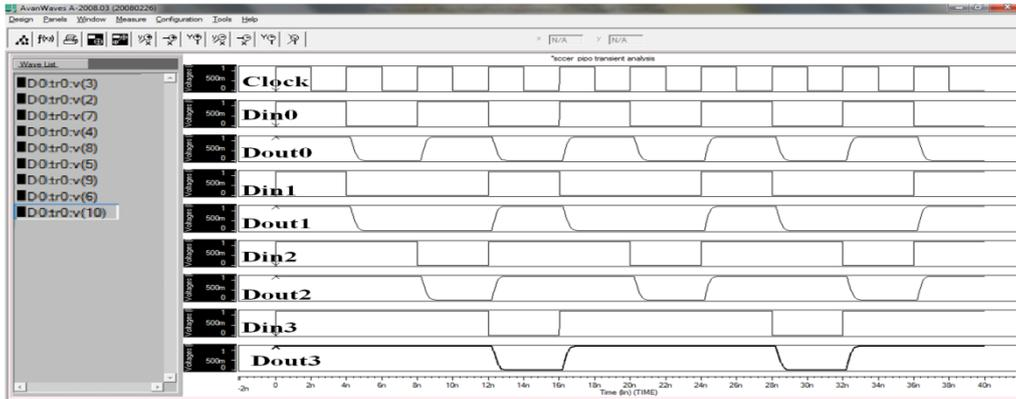
Fig 23. Output of parallel-in and parallel-out shift register using SCCER flip-flop.
