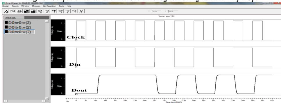
Fig 16 Output of serial-in and serial-out shift register using SCCER flip-flop.
