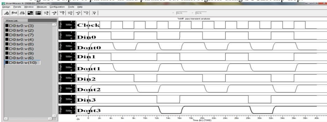
Fig 24. Output of parallel-in and parallel-out shift register using MHLFF flip-flop.
