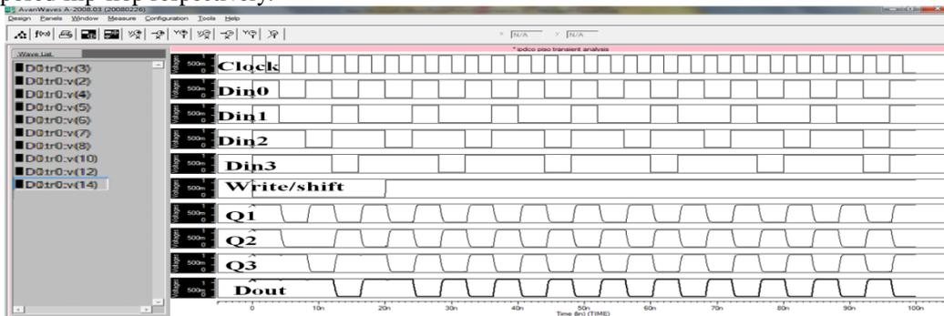
Fig 26. Output of parallel-in and serial-out shift register using IP-DCO flip-flop.
