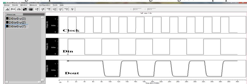
Fig 17. Output of serial-in and serial-out shift register using proposed flip-flop.
