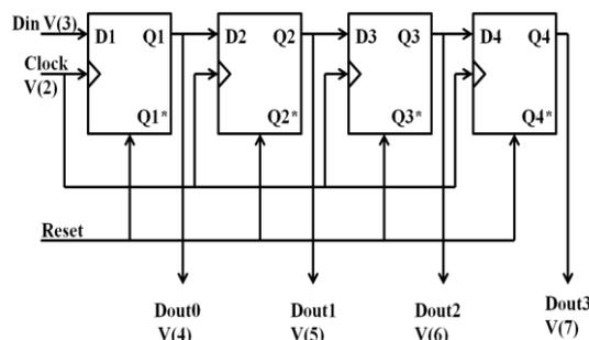
Fig 7. Serial-in and parallel-out shift register.
