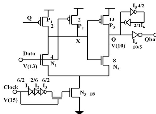
Fig. 3 Circuit diagram of Modified Hybrid Latch Flip-flop.
