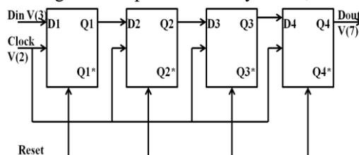
Fig 6. Serial-in and Serial-out shift register.
