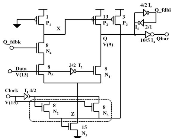
Fig. 5. Circuit diagram of the proposed P-FF design with pulse control scheme.
