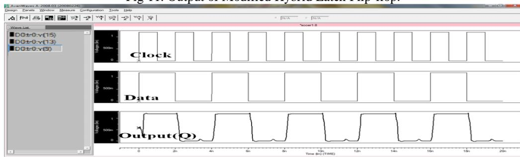
Fig 12. Output of SCCER Flip-flop.
