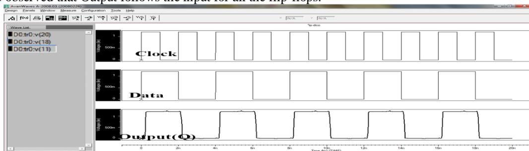
Fig. 10 Output of IP-DCO Flip-flop.
