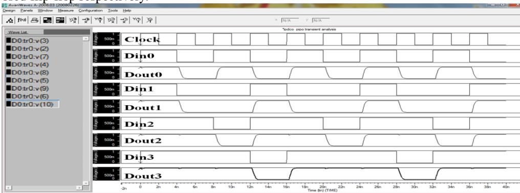
Fig 22. Output of parallel-in and parallel-out shift register using IP-DCO flip-flop.
