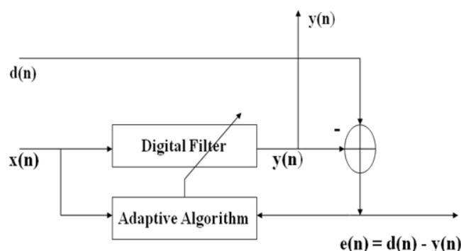
Fig2: Block diagram of Adaptive Filter [4].
