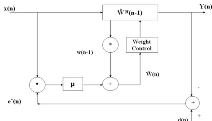
Fig3: Block diagram of LMS Algorithm [13].
