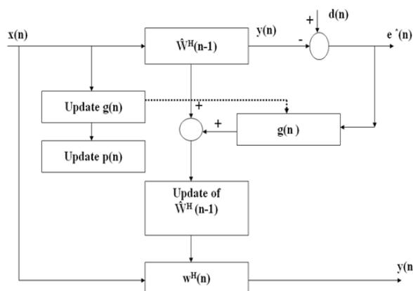
Fig4: Block diagram of RLS Algorithm [13].
