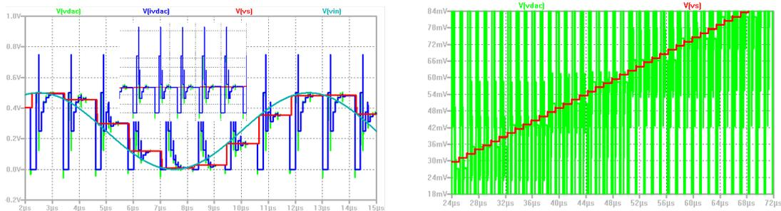
Figure 12: Transient Simulation of ADC
