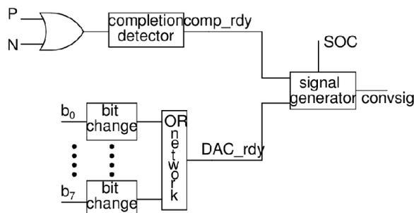
Figure 10: SAR Controller signal generation scheme
