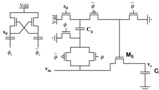
Figure 2: Sample/Track and Hold Circuit
