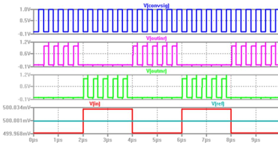
Figure 5: Comparator Transient Simulation
