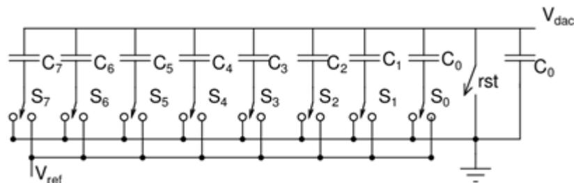
Figure 6: DAC Circuit
