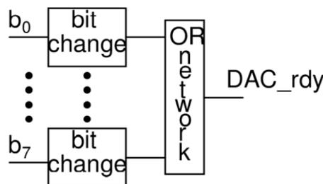
Figure 8: DAC completion detection scheme
