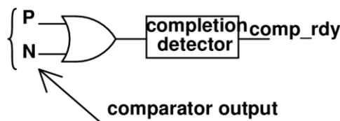
Figure 9: Comparator completion detection scheme
