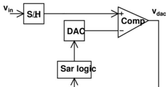
Figure 1: ADC Block Diagram
