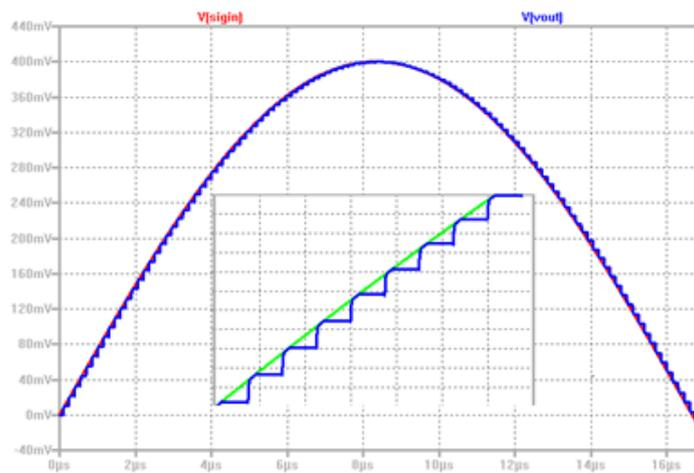
Figure 3: Sample/Track and Hold Transient Simulation
