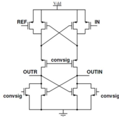
Figure 4: Comparator Circuit
