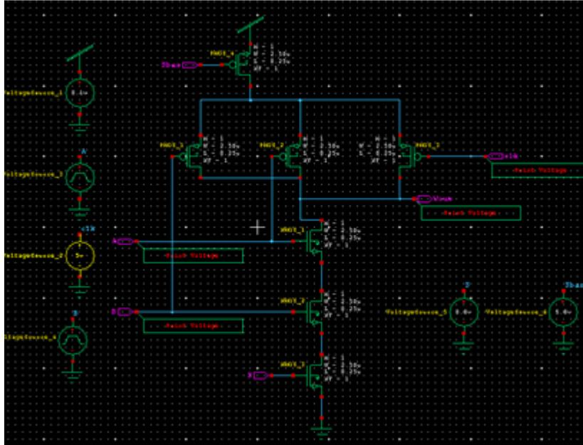
Figure 7: Schematic of Type A Static NAND gate with Sleep Power Gating
