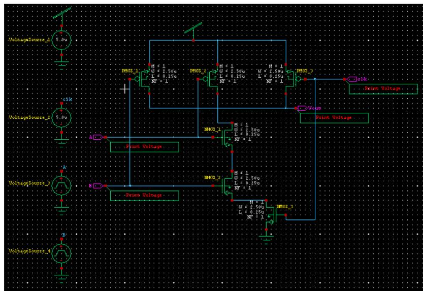
Figure 2: Schematic of Type A Static NAND gate
