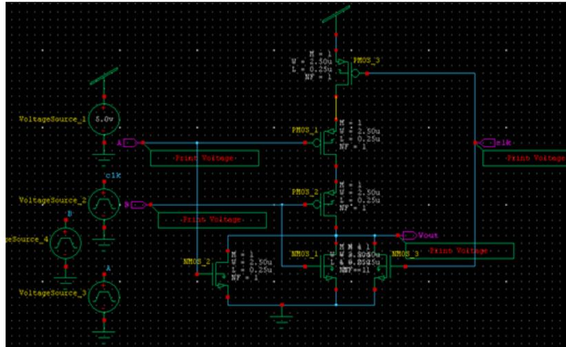
Figure 3: Schematic of Type B Dynamic NOR gate
