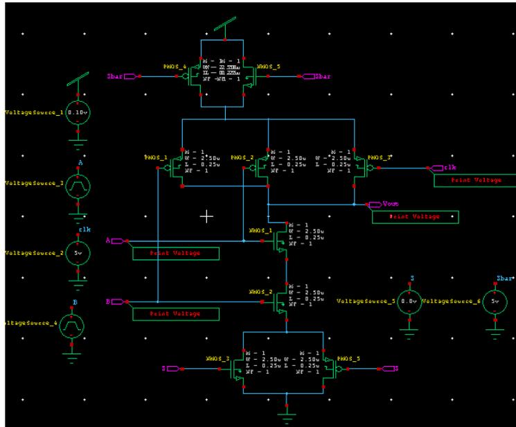
Figure 9: Schematic of Type A Static NAND gate with Dual Sleep Power Gating
