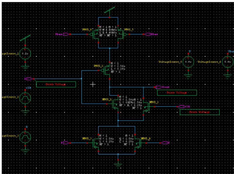
Figure 8: Schematic of Type B Dynamic NOT gate with Sleepy Stack Power Gating
