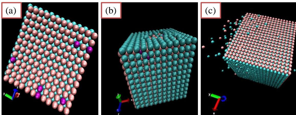
**Figure 9:** Final film structure at  $20Ps$  (a) Ni-Ti-Cu, (b) Ni-Ti, (c) Ni-Cu.
