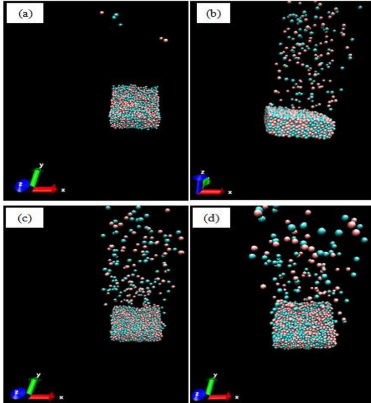
**Figure 10:** Film Structure of resputtering process started as the negative substrate bias voltage is increasing at different time intervals (a) for time  $t = 5Ps$ , (b) for time  $t = 10Ps$ , (c) for time  $t = 15Ps$ , (d) for time  $t = 20Ps$ .
