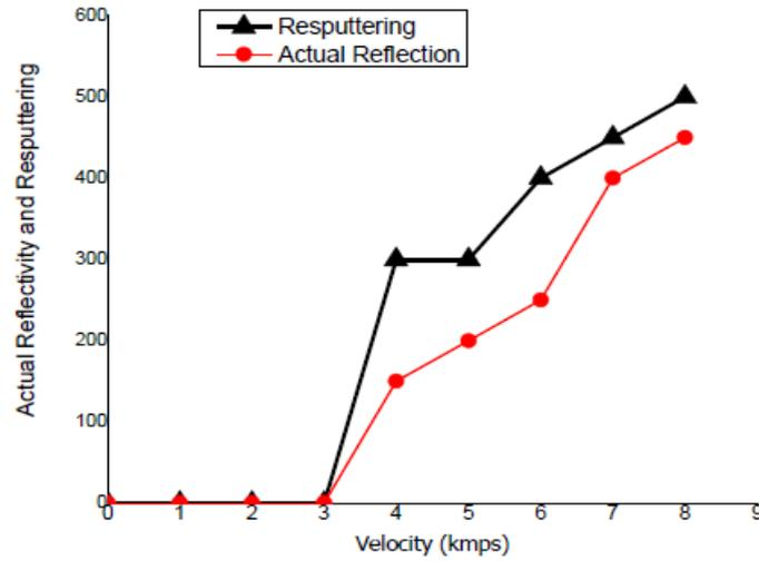
Figure 5: Variation of number of atoms which have been reflected and re-sputtered with colliding velocity.
