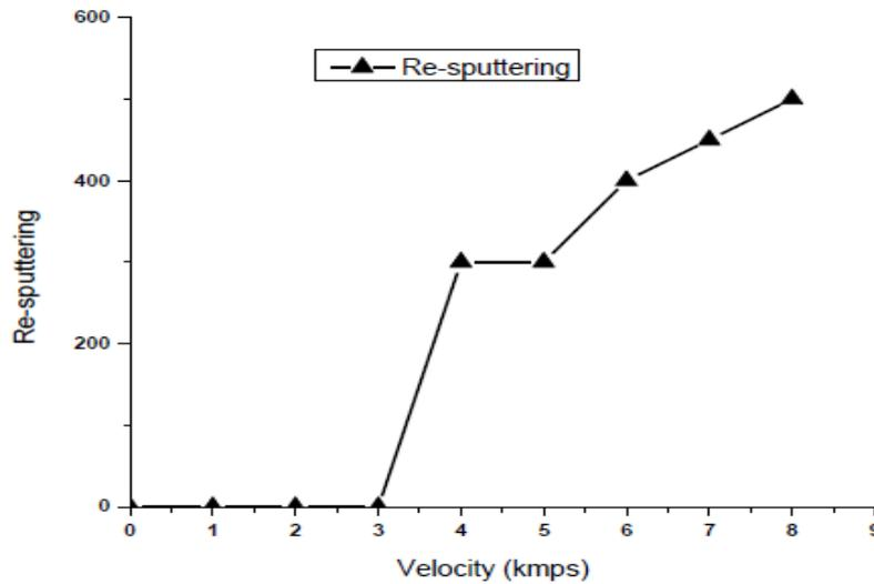
Figure 6: Variation of number of atoms which have been reflected with colliding velocity.
