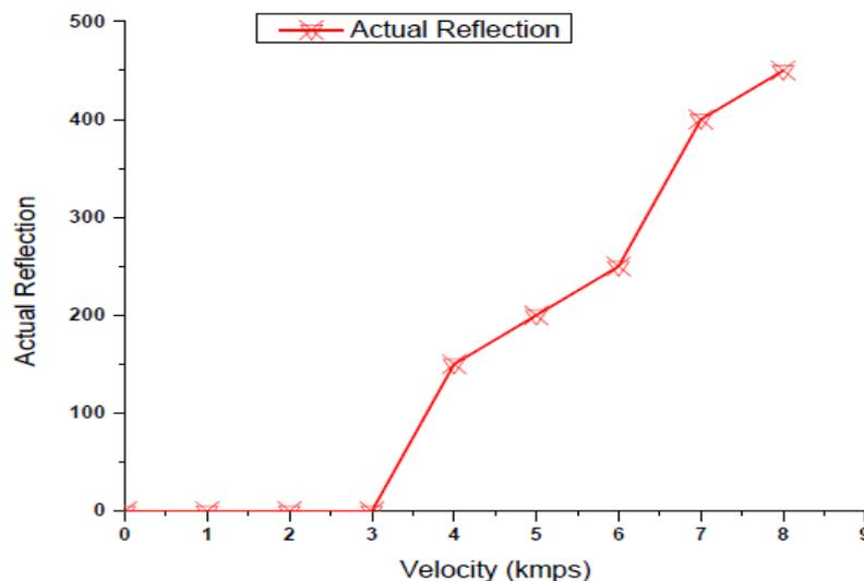
Figure 7: Variation of number of atoms which have been re-sputtered with colliding velocity.
