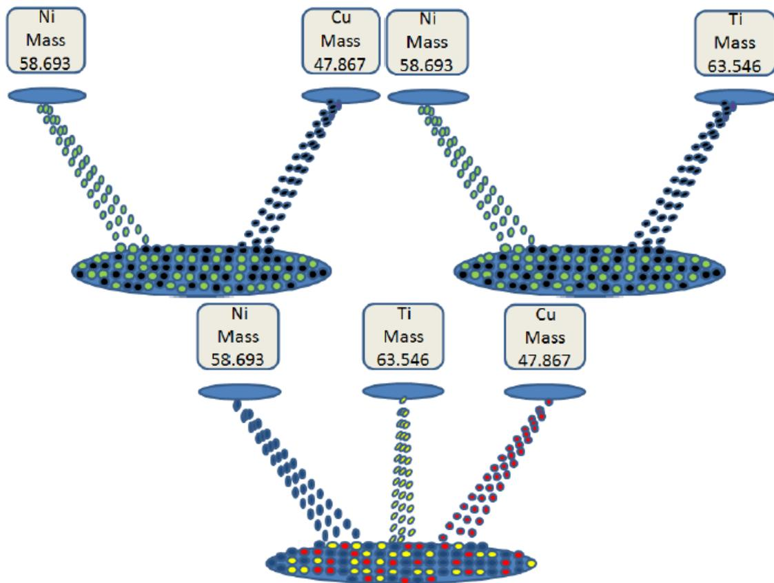
**Figure 4:** The schematic structure represents the Ni, Ti and Cu atoms striking a representative portion of Ni-Ti, Ni-Cu and Ni-Ti-Cu thin film.
