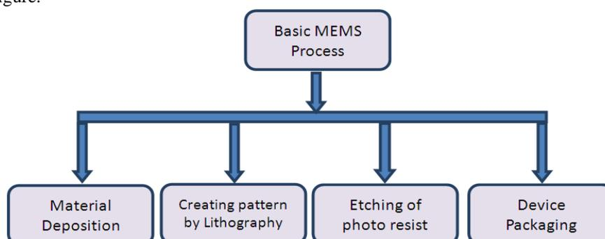
Figure 1: Flow chart of MEMS fabrication process.
