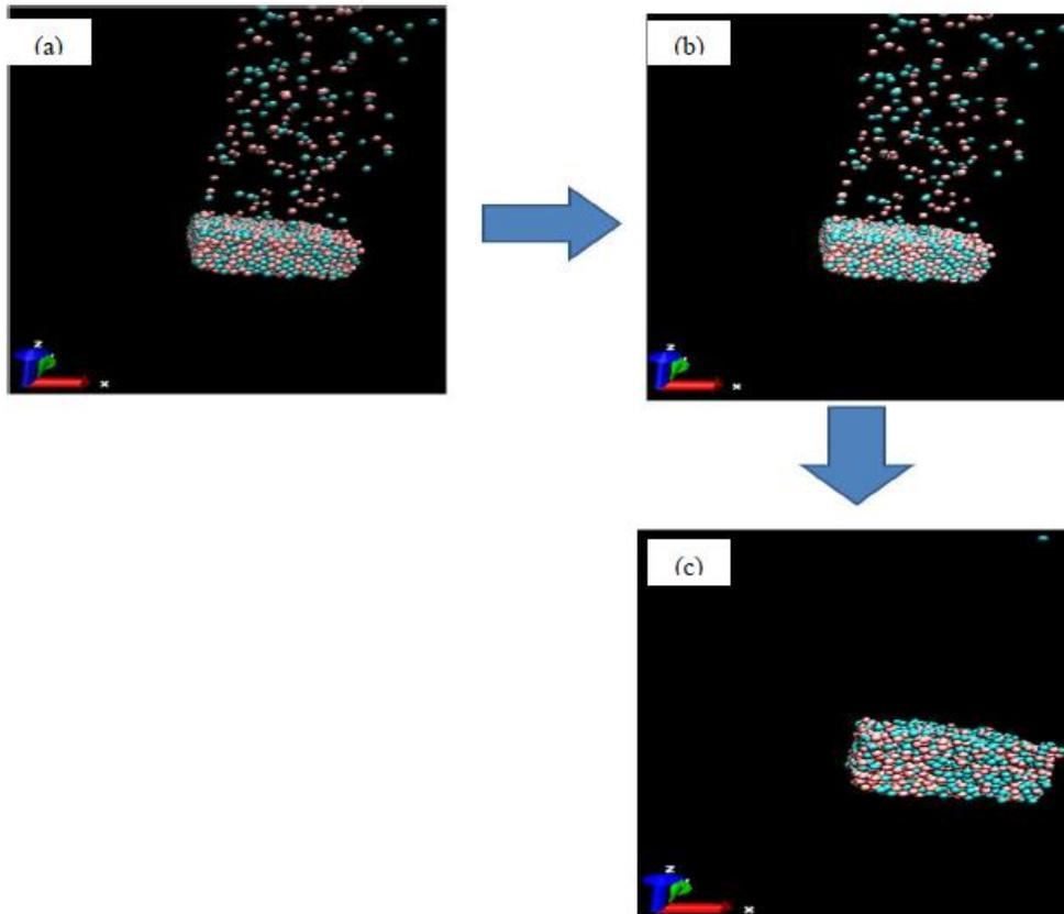
**Figure 8:** The development of the thin film at different time intervals (a) for time  $t = 10Ps$ , (b) for time  $t = 15Ps$ , (c) for time  $t = 20Ps$ .
