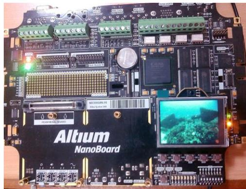
Fig 3: Histogram Equalized Image on Altium NB3000TFT
