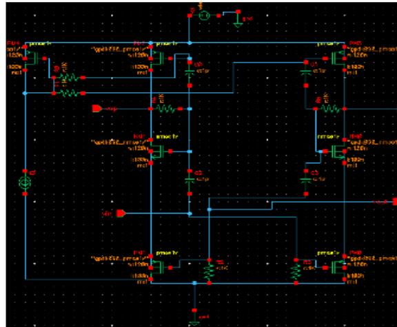
Fig 1. Broadband LNA with resistive feedback
