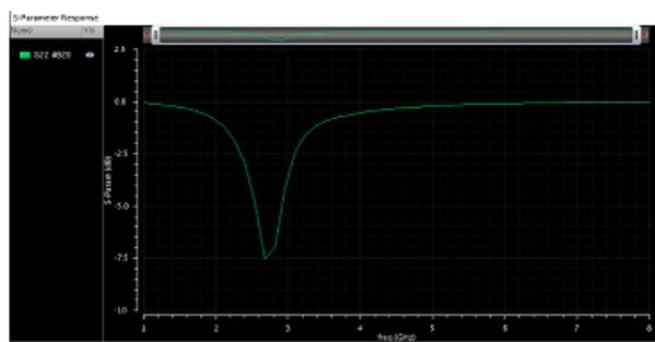
Fig 7.  $S_{22}$  Output Reflection Coefficient
