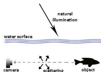
Fig.2 Underwater image acquisition
