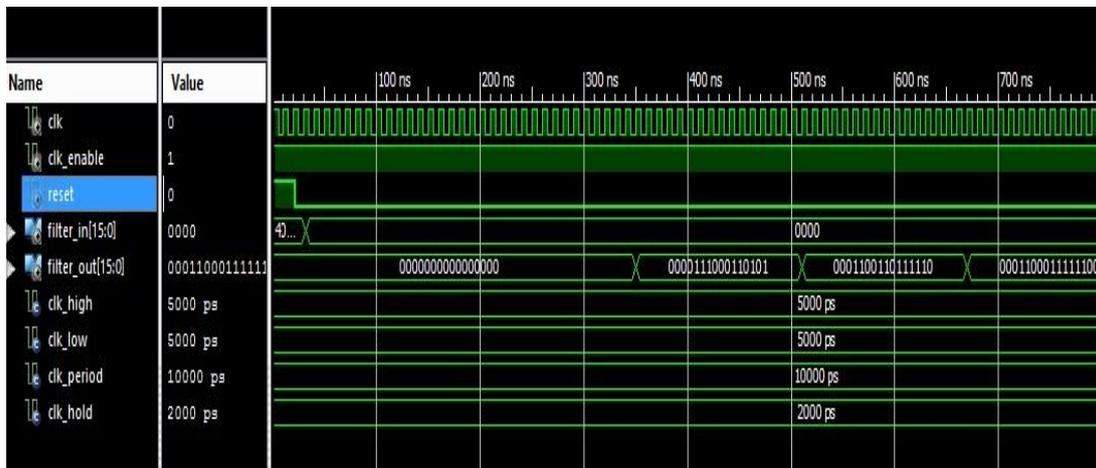
Fig. 8 Simulation waveform NLMS Adaptive filter 20 coefficients.
