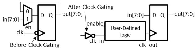
Fig. 2. Gating the clock input
