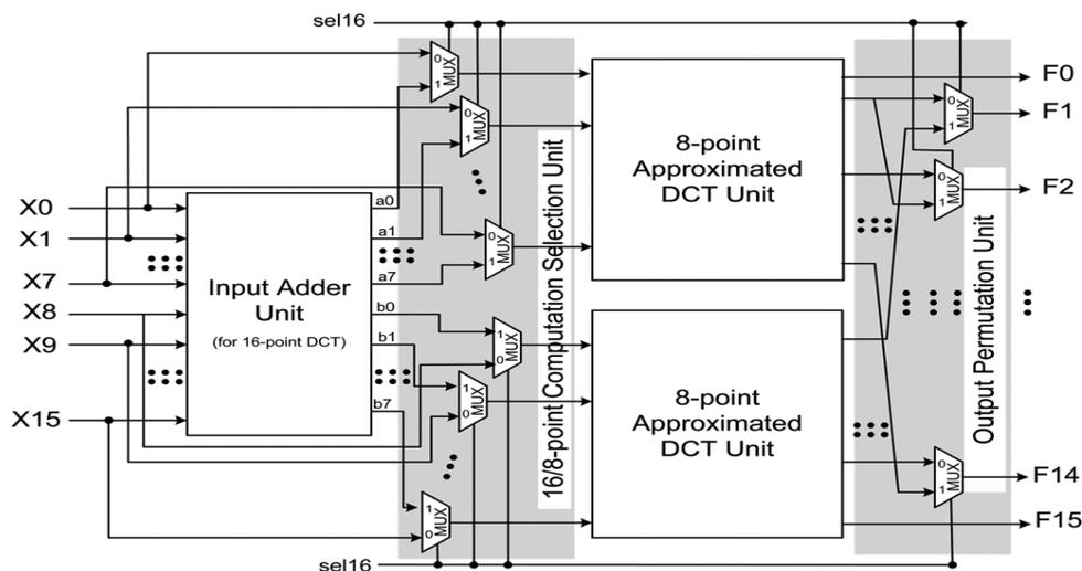
**Fig. 4** Proposed reconfigurable architecture for approximate DCT of lengths  $N = 8, 16$  and  $32$ .
