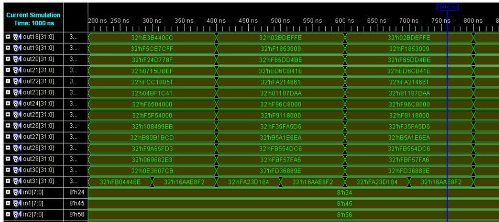
Fig. 7 32-point DCT output
